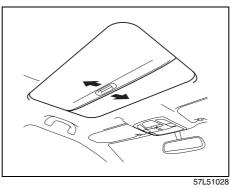
To slide the sunroof rearward, push the "SLIDE OPEN" part (2) of the sunroof switch. To slide the sunroof forward, push the "TILT UP" part (1) of the sunroof switch.
